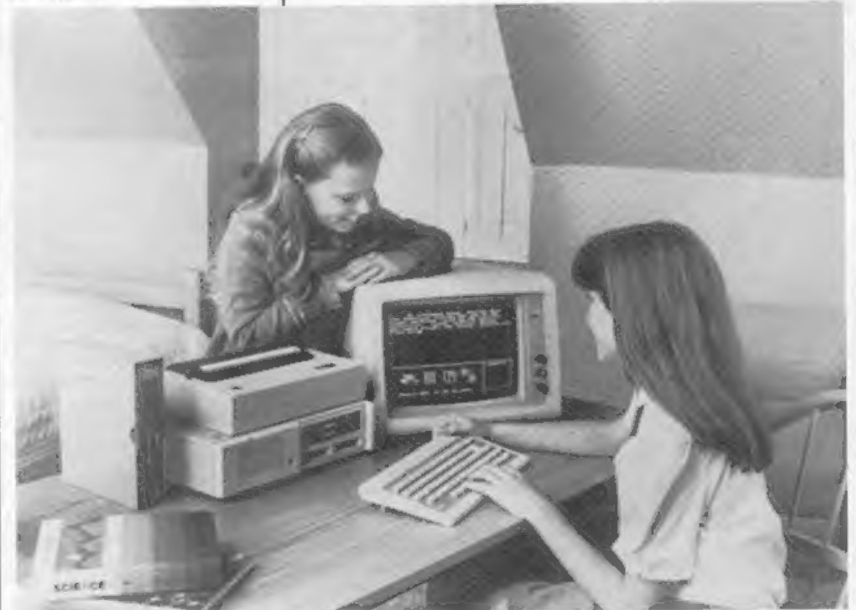
IBM's PC Junior with the thermal printer perched on top of the main unit
